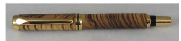
Needed: Mandrel-A Bushings-19A Drill-15/32" & 25/64" Wood Size- <sup>3</sup>/4" x <sup>3</sup>/4"
